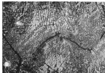
Fig. 7 – Area affected by cavitations with a micro cracks, detachments and grain expulsions – OM 500×.
