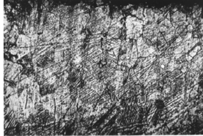
Fig. 8 – Area affected by cavitations with a grain finish and complex precipitation – OM 500×.
