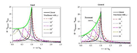
Fig. 4.2 – Magnification functions for cohesionless soils.
