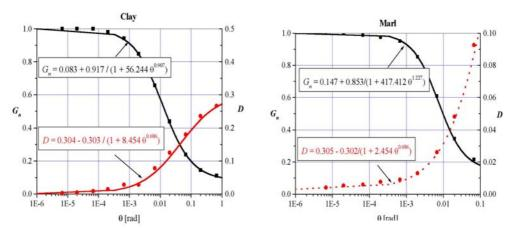
Fig. 2.1 – Dynamic functions for cohesive soils.
