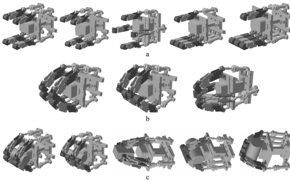
Fig. 12 – Modular anthropomorphic gripper with four fingers.
