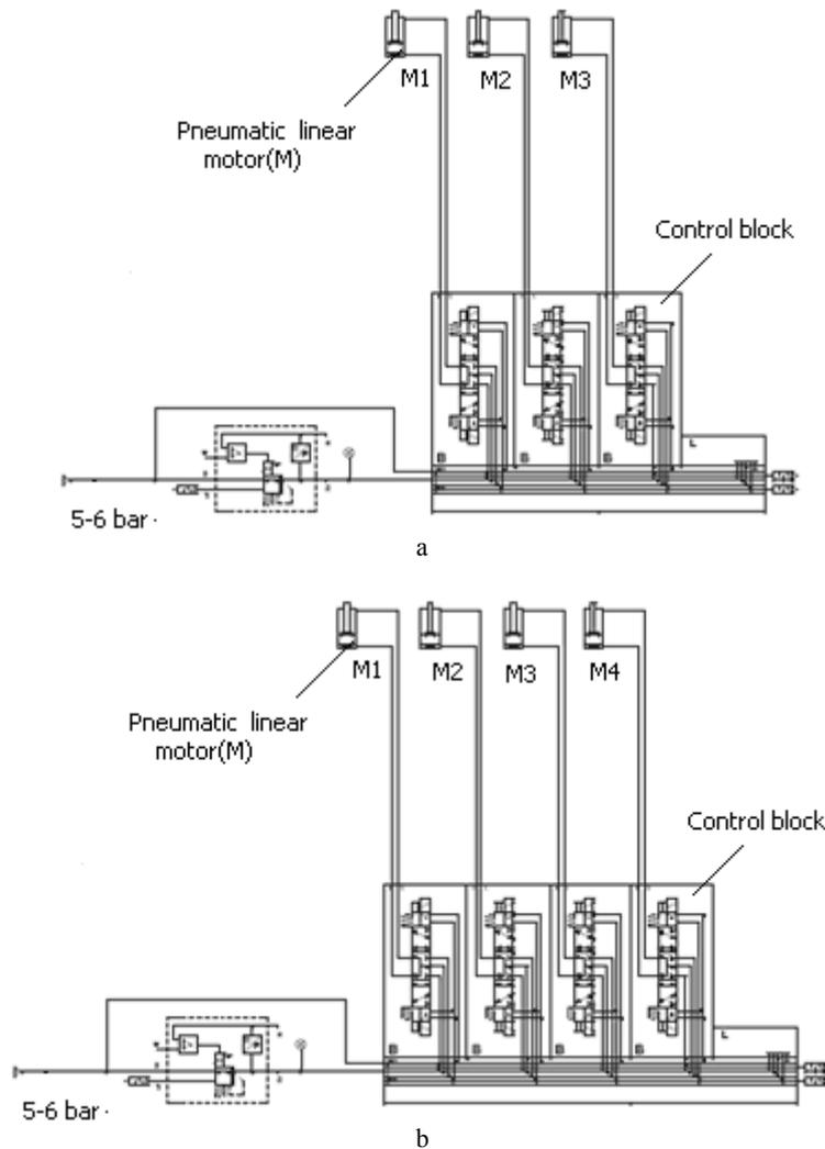
Fig. 16 – Actuated pneumatic scheme.
