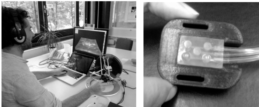
Fig. 4 – Palpation Feedback realized with five small balloons in an epoxy matrix actuated by compressed air. This device was mounted on an the OMEGA handle and used for finding a hidden artery in the piece of Virtual Reality (VR) soft tissue represented on the computer screen.
