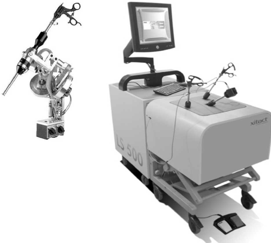
Fig. 6 – Simulator for laparoscopic surgery with force feedback (xitact SA, Morges).
