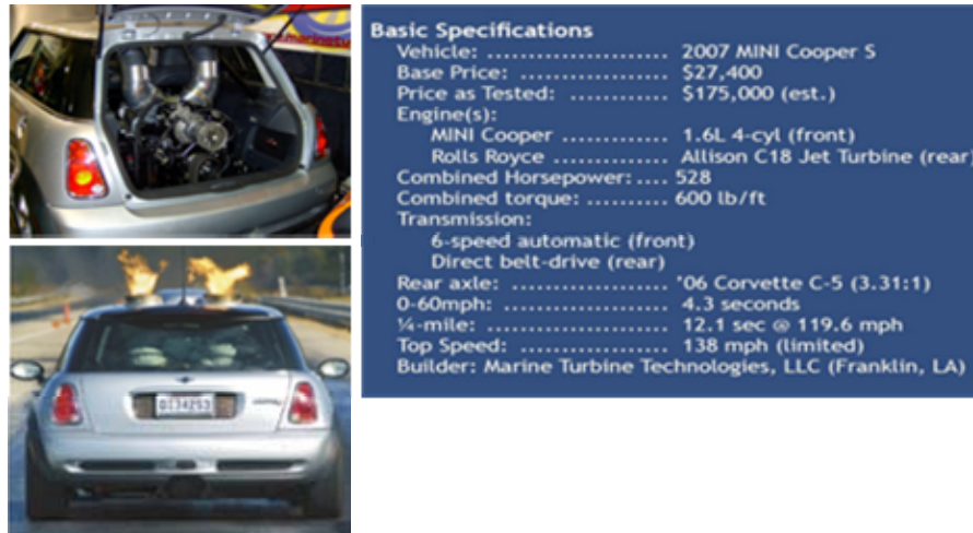
Fig. 8 – MINI Cooper S with propulsion by gas turbine (rear) and piston engine (front).
