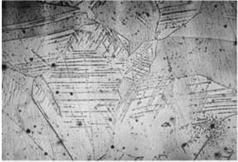
Fig. 1 – The microstructure of the steel GX5CrNi19-10 after Heat Solution Treatment: 1050 °C / 30 minutes/water; OM 500×.
