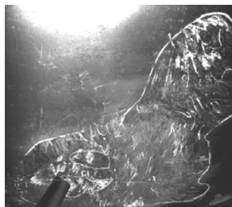
Erosion on the suction side of the blade (Stainless steel OH12NDL)
