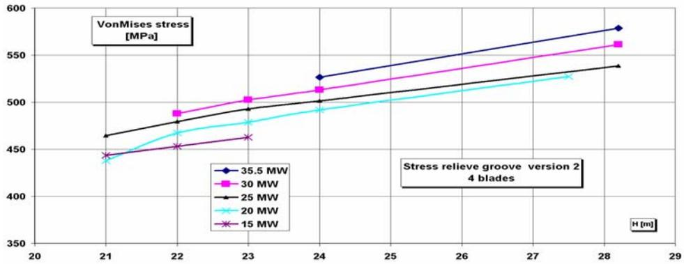
Fig. 11 – The Von Mises stress for stress relieve groove version 2, 4 blades.
