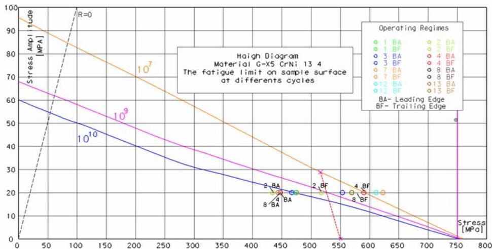
Fig. 13 – The Haigh diagram for stress relieve groove version 1 and 4 blade.
