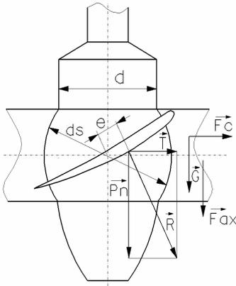
Fig. 4 – The theoretical blade loads
