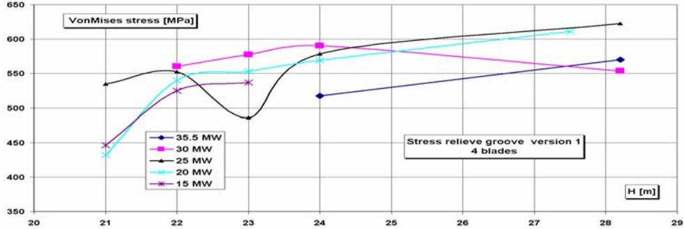
Fig. 10 – The Von Mises stress for stress relieve groove version 1, 4 blades.
