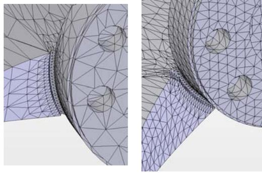
Fig. 7 – The blade mesh in the stress relieve groove area version 1 / version 2.
