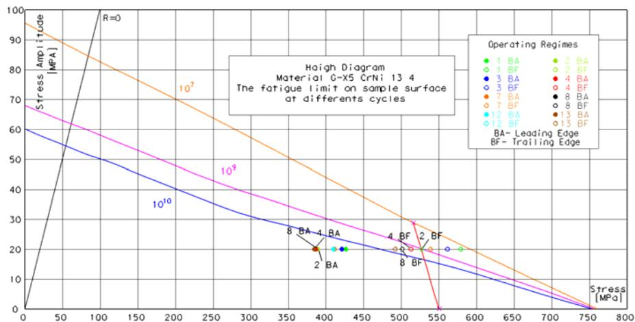
Fig. 14 – The Haigh diagram for stress relieve groove version 2 and 4 blade.
