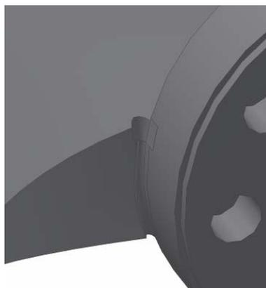
Fig. 3 – The geometry of the stress relieve groove – version 2.
