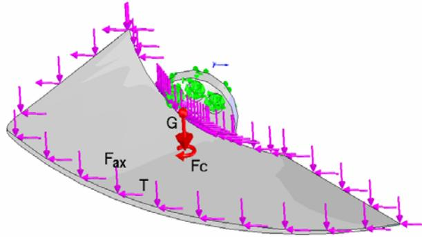
Fig. 5 – The blade loads applied in Design Star.
