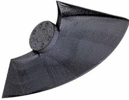
Fig. 6 – The blade mesh.
