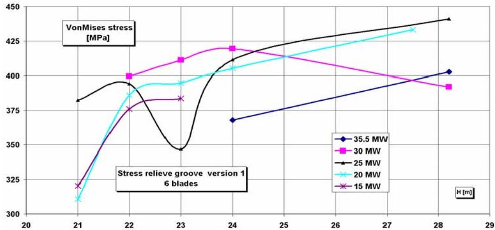
Fig. 12 – The Von Mises stress for stress relieve groove version 1, 6 blades.
