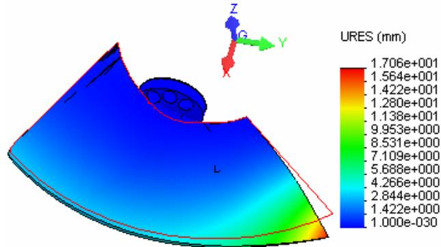
Fig. 8 – The resultant displacement plot.
