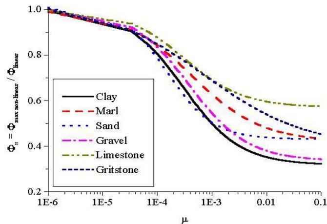
Fig. 4.4 – Resonant curves in normalized form.
