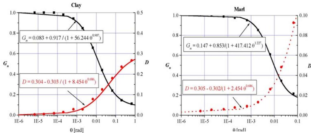
Fig. 2.1 – Dynamic functions for cohesive soils.
