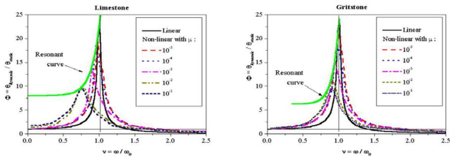
Fig. 4.3 – Magnification functions for rocks.
