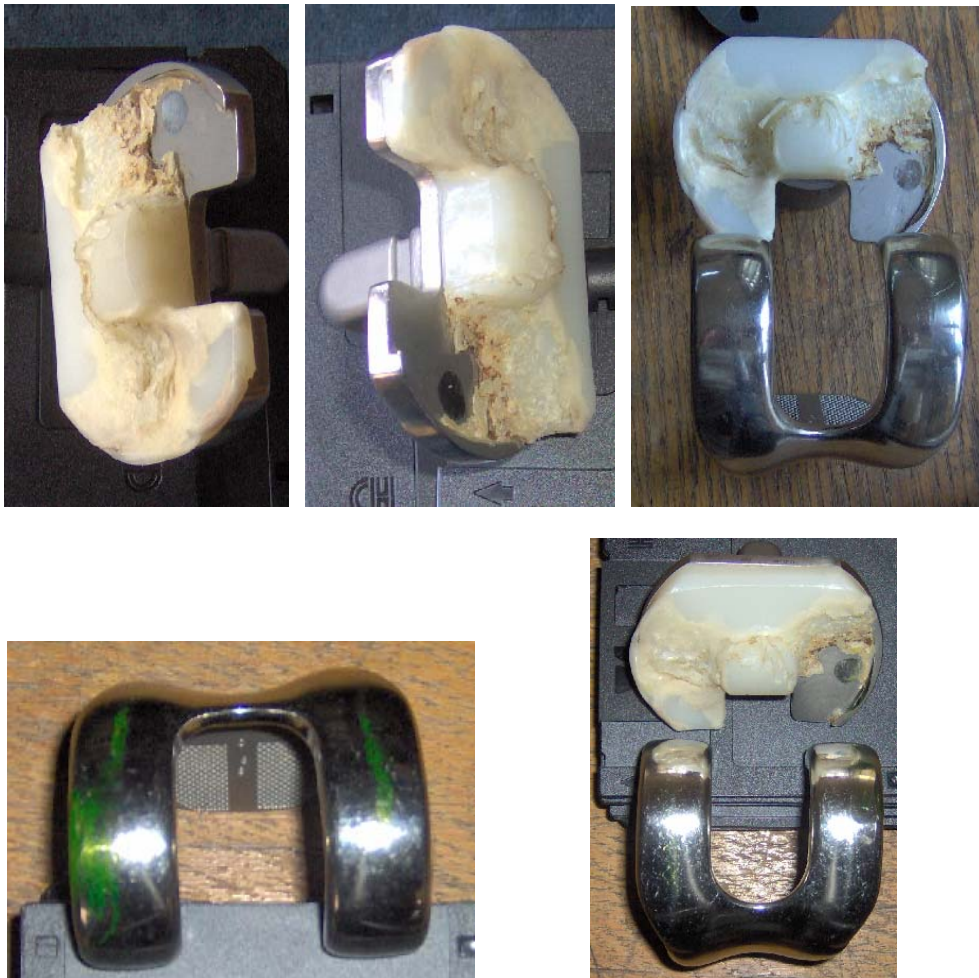
Fig. 1 – Images of the total knee prosthesis components with fatigue wear.
