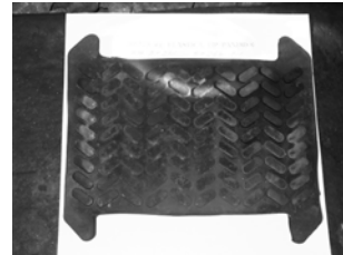
Fig. 3 – PANDROL fixing type using rigid grips and deformed PR3 plate.
