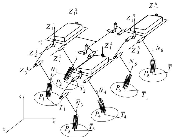
Fig. 2 – Mathematic modelling of the gravity centre position.
