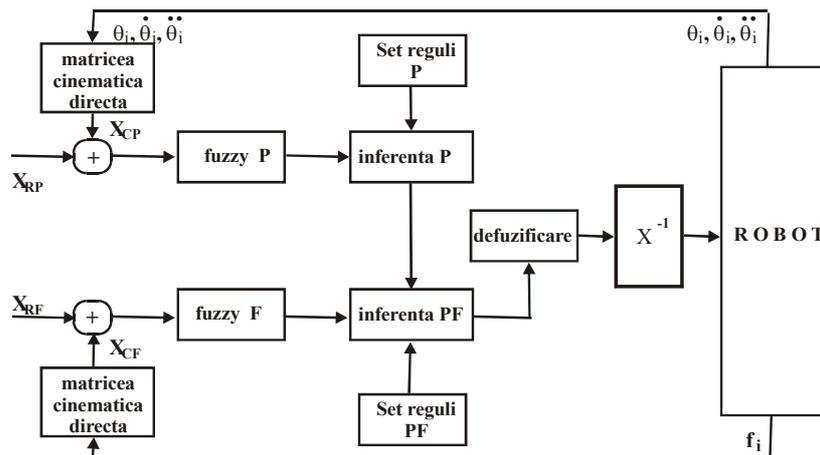
Fig. 5 – Fuzzy multi-stage control (FMS) for tracking processes.
