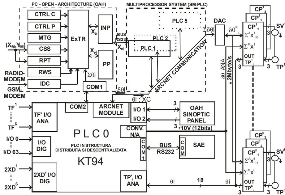
Fig. 8 – Real time control system with open architecture for the MERO modular walking robot.
