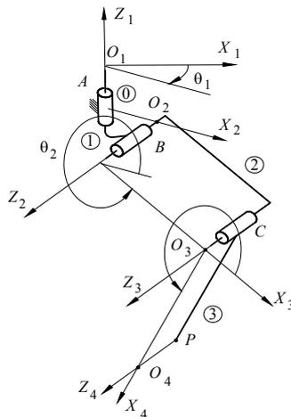
Fig. 1 – Kinematics modelling of the leg's mechanisms.
