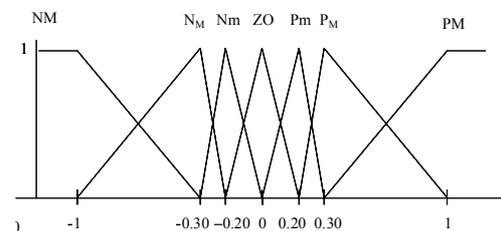
Fig. 7 – Rate error input fuzzy sets.
