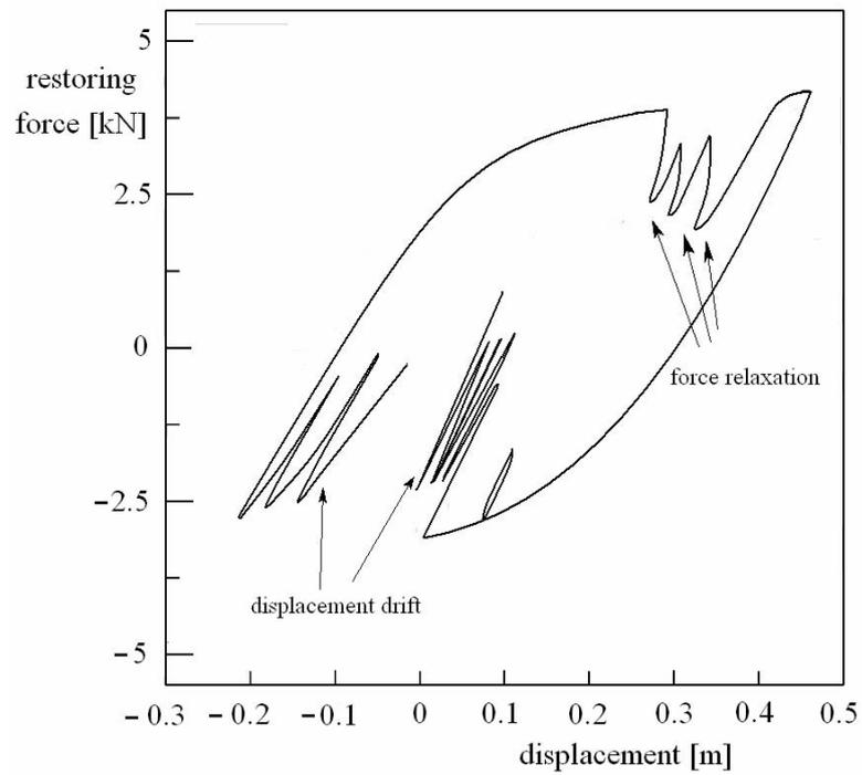
Fig. 11 – The displacement drift and force relaxation.
