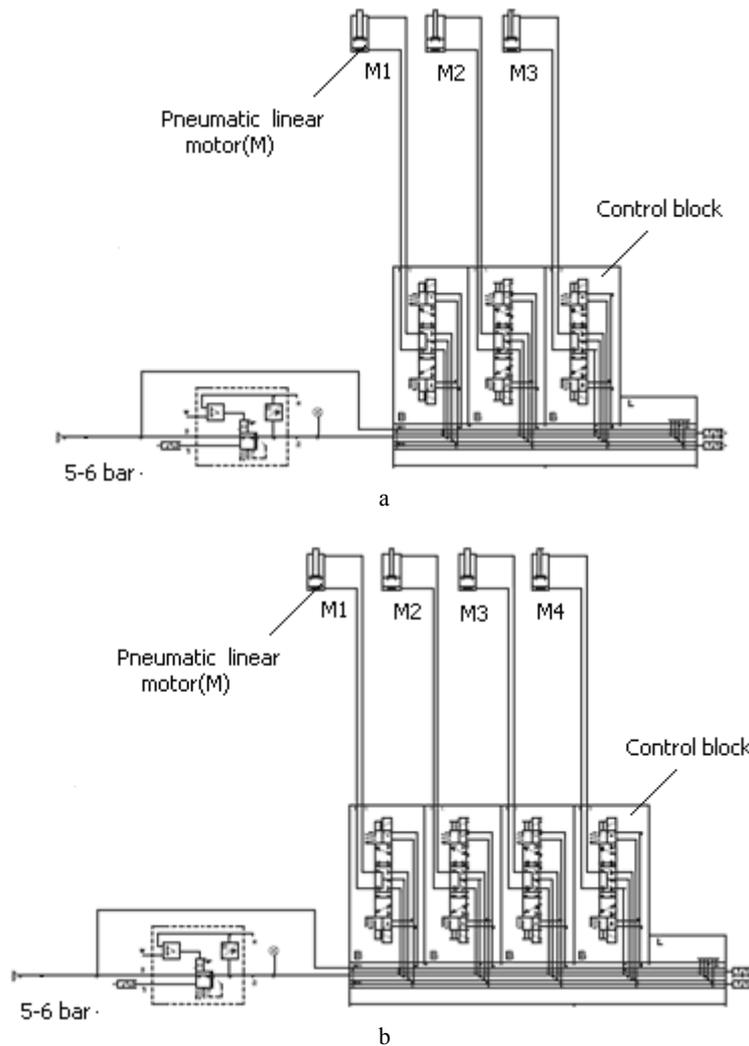
Fig. 16 – Actuated pneumatic scheme.
