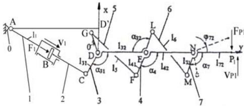
Fig. 4 – The structural scheme of the finger.
