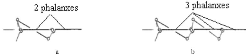
Fig. 2 – Fingers with two phalanxes (a) and three phalanxes (b).
