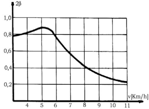
Fig. 2 – The diagram of the variation of the 2\beta factor as a function of velocity, for the collision of two vehicles equipped with 75 mm buffers (case 1).
