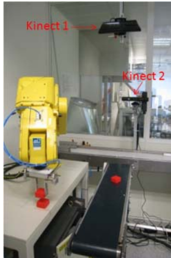
Fig. 12 – Low cost 3D vision system.
