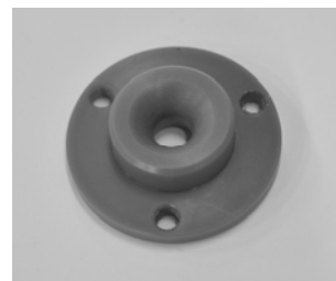
Fig. 19 – Movable die used in experiments.
