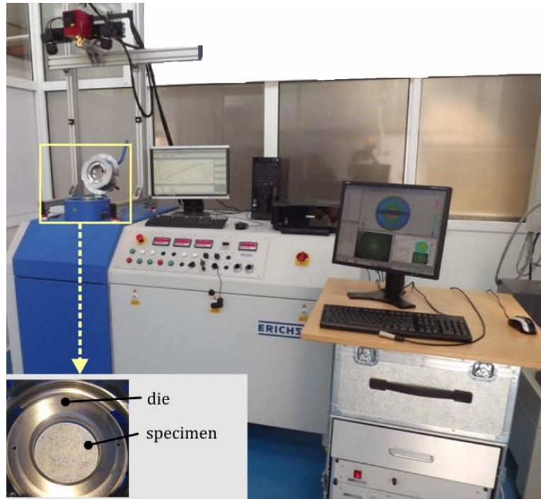
Fig. 2 – Experimental stand consisting in the ERICHSEN bulge test device and the ARAMIS 3D.
