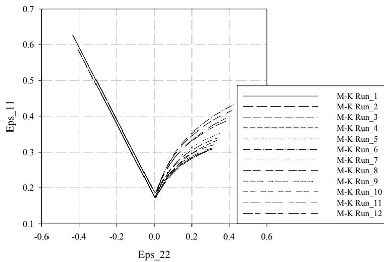
Fig. 6 – Forming limit curves obtained by varying the mechanical parameters for BBC2005 yield criterion and M-K model.
