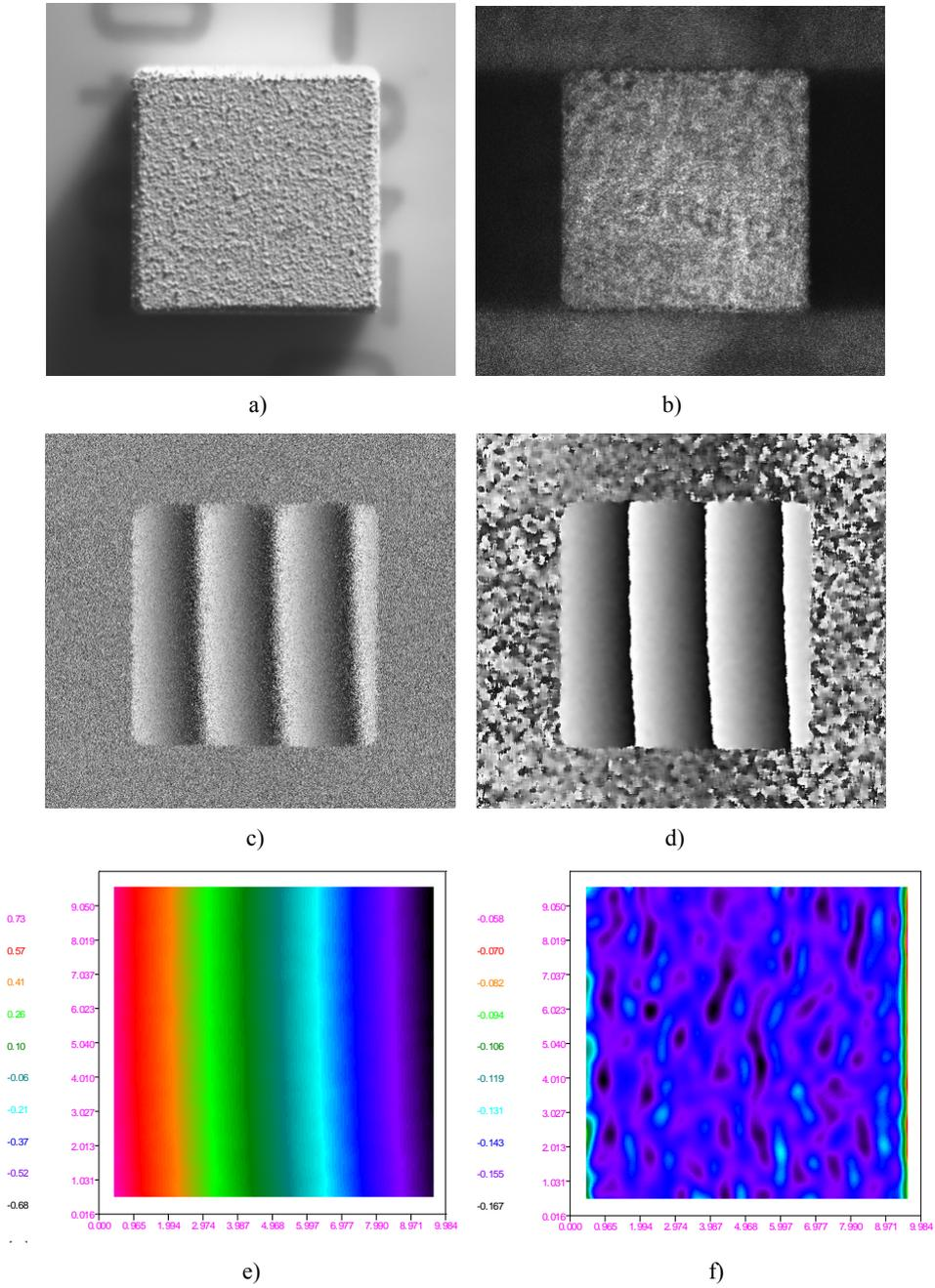
Fig. 4 – Thermal expansion of an aluminium sample measured by ESPI:
