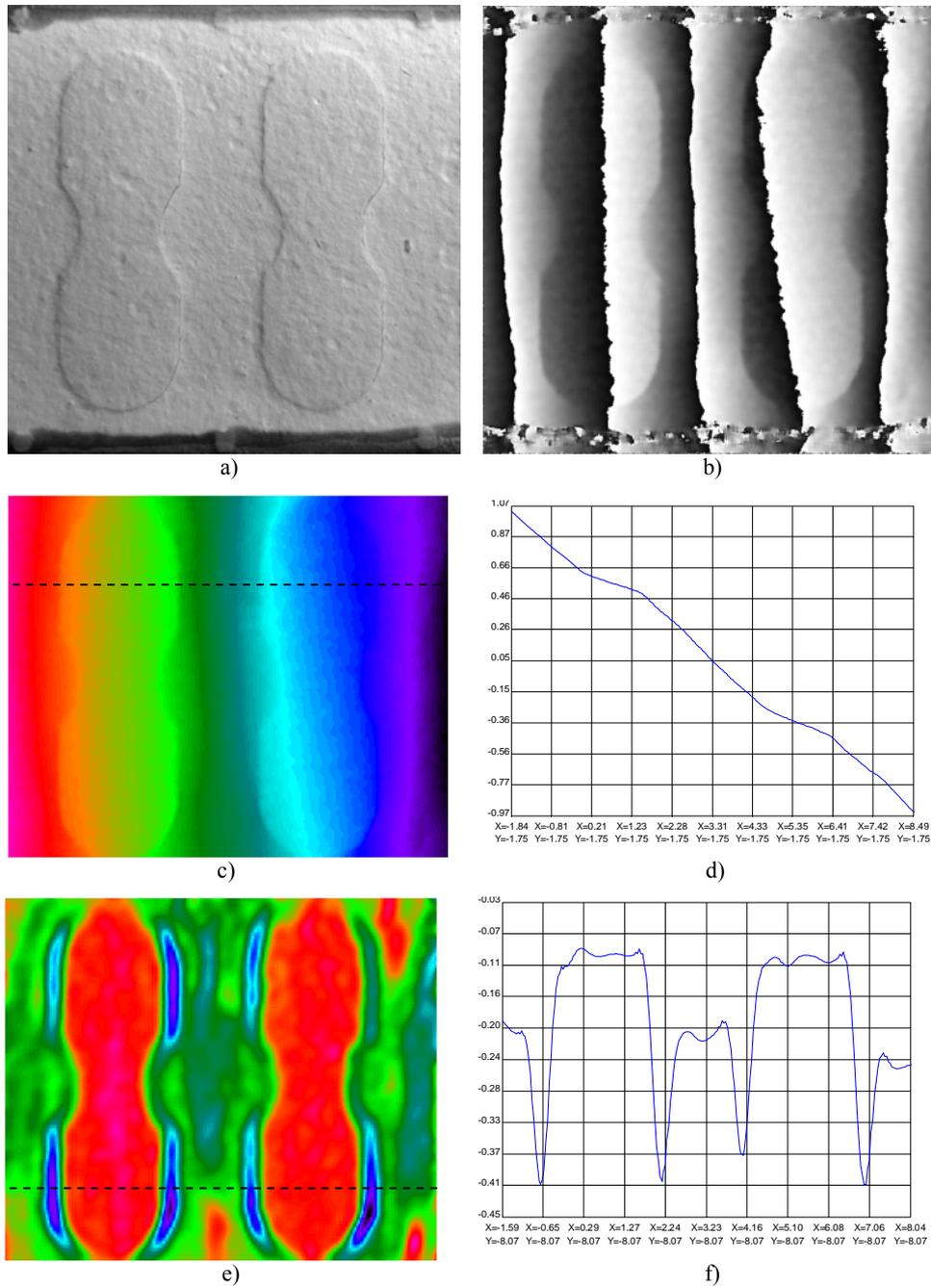
Fig. 4 – Thermal expansion of a layered foil of different materials measured by ESPI: a) sample view; b) filtered phase map; c) displacements ( $u_x$ ); d) horizontal profile of displacements; e) strains ( $\epsilon_x$ ); f) horizontal profile of strains.
