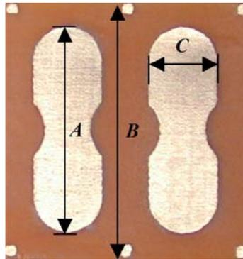
Fig. 1 – Thin foil specimen: strain gauge solder terminal.
