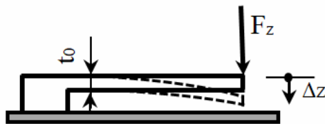
Fig. 2 – Free-end beam. The beam bends under the action of the force in z -direction.
