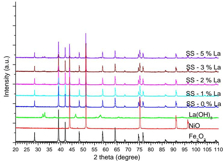
Fig. 2 – X-ray diffraction patterns of the starting mixtures (0, 1, 2, 3 and 5 % La),  $\text{La(OH)}_3$ , NiO and  $\text{Fe}_2\text{O}_3$ .
