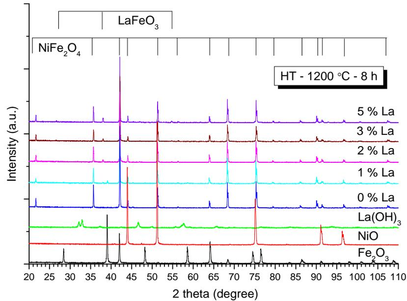
Fig. 6 – X-ray diffraction patterns of the samples heat treated (HT) at 1 200 °C for 8 h in air. For reference are given the X-ray diffraction patterns of the  $\text{La(OH)}_3$ ,  $\text{NiO}$  and  $\text{Fe}_2\text{O}_3$ .
