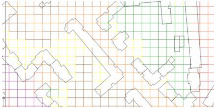
Fig. 11 – Detail view of the noise level grid around buildings.
