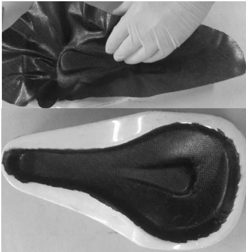
Fig. 9 – Application of CFRP layers on the mold.
