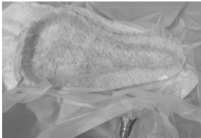
Fig. 10 – Applying vacuum pressure through mold and composite material.
