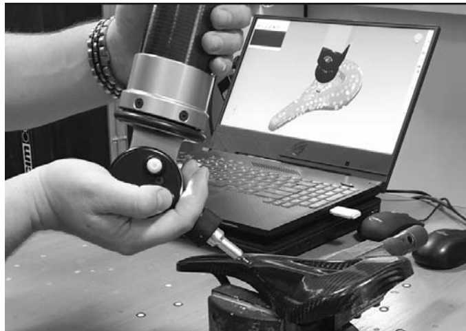
Fig. 13 – Dimensional evaluation of CFRP seat post.
