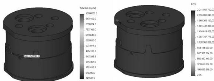
Fig. 13 – Total life-cycle and safety factor estimated by the SolidWorks simulation program.
