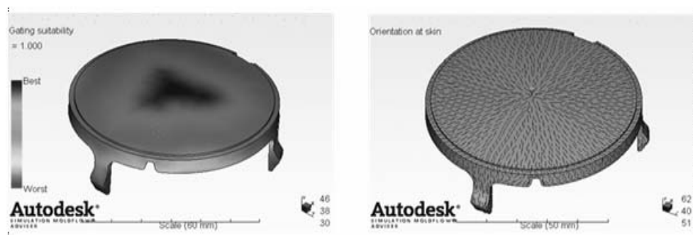
Fig. 6 – Optimal gate location and fiber orientation (Moldflow).
