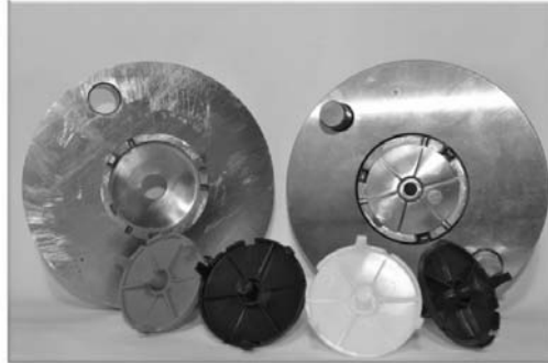
Fig. 18 – Tooling plates and tooling inserts made by SLM at TUCN mounted onto the plates.
