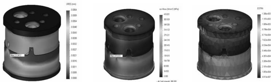
Fig. 11 – Results obtained from the static analysis (SolidWorks simulation).
