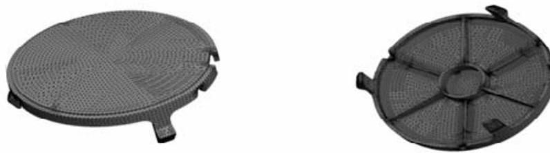
Fig. 5 – Mesh details (MoldFlow).
