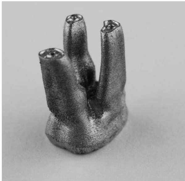
Fig. 9 – Manufactured mandibular first molar using SLM process.
