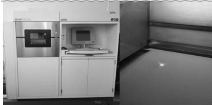
Fig. 1 – EOSINT M270 Dual Mode Machine, owned by INCDMTM and the laser beam.
