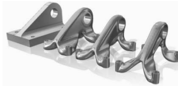
Fig. 6 – Topological optimization of a virtual model, www.solidedge.siemens.com .
