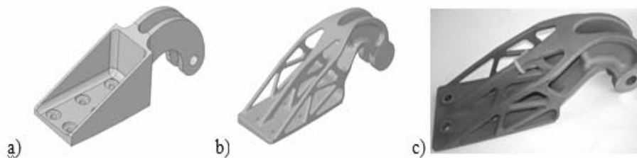
Fig. 4 – Engine nacelle hinge from Airbus: a) conventional design; b) redesigned for AM; c) SLM-manufactured [18].
