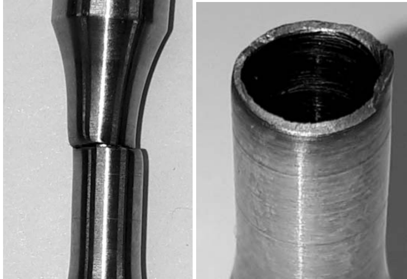
Fig. 9 – Specimen failed by proportional tension-torsion fatigue test.
