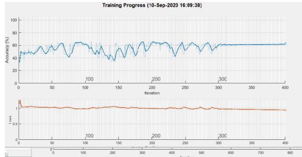
Fig. 17 – Accuracy estimation during training for a LSTM applied on Fourier power spectra.
