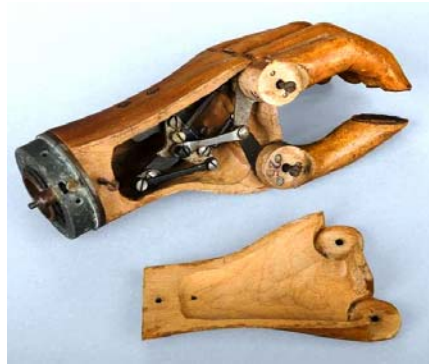
Fig. 1 – Hand prosthesis with fingers motion mechanism (1920) [1].
